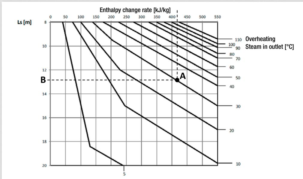
Fig. 6: Distance between desuperheater and temperature sensor
