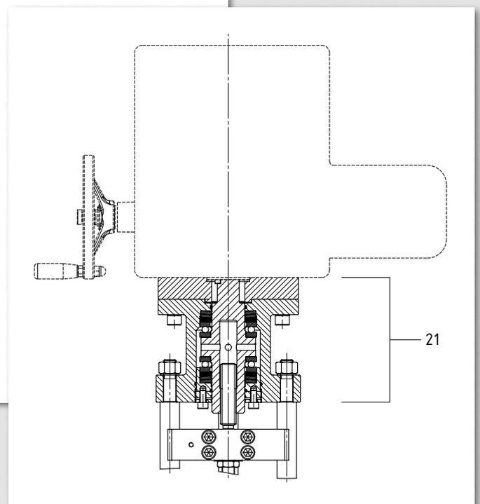
Fig. 11: Gearbox (electric actuator)
