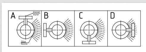
Fig. 4: Water connection flange options
