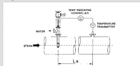
**Fig. 6: Distance between Desuperheater and Temperature Sensor**
