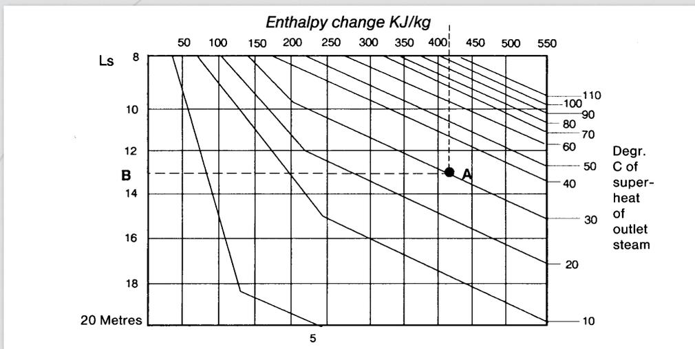
\*Above values are for DN 300 pipe sizes for other pipe sizes multiply distance by  $0,06 \sqrt{D}$  (D = pipe dia.)
