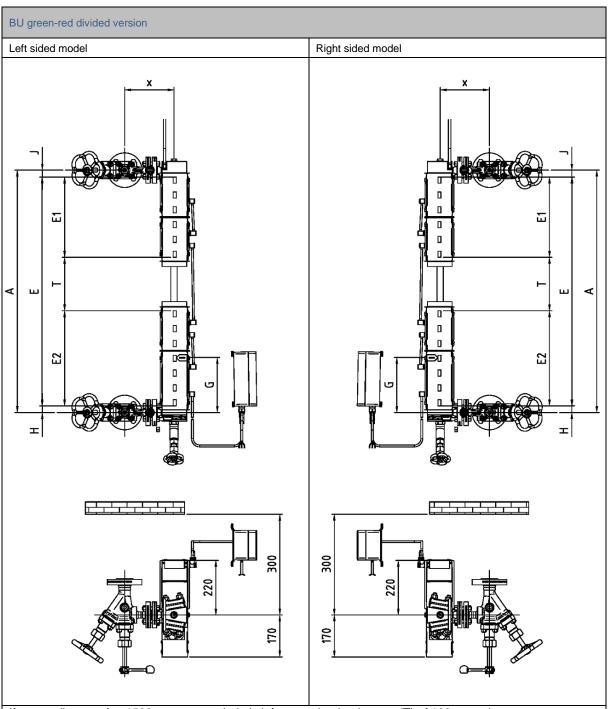
If center distance A > 1530 mm one porthole is left out and a dead space (T) of 100 mm arises. The position of the dead space depends on the order
