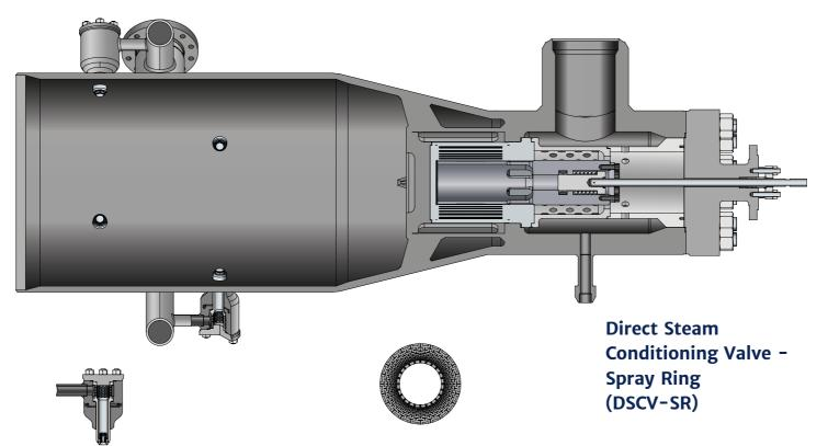
spacer has been specifically designed to negate any upstream pipe work induced flow disturbance being communicated to the main plug. Therefore, long radius bends or isolation valves can be fitted directly to the valve inlet to minimize installation space. The main plug is fully guided by the cage and spacer to ensure complete plug stability through full travel.
