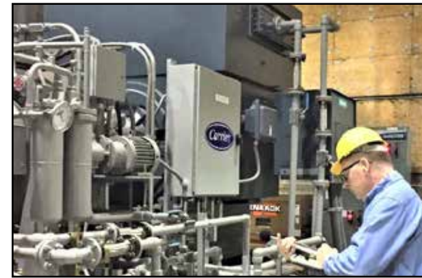
SOUND PRESSURE LEVEL MEASUREMENTS - AHRI-575 TEST METHOD
